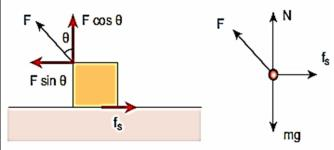
From the diagram the normal force N is balance by the total downward force mg - Fcosθ. Thus,
