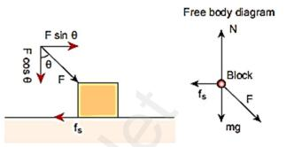
From the diagram the normal force N is balance by the total downward force mg + Fcosθ. Thus,
