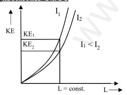
The graph shows that of the two bodies of same angular momentum, those one have less rotational kinetic energy has higher moment of inertia.
