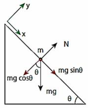
As the normal force N is compensated by mgcos $\theta$ , there is no motion along y-axis.
