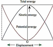
In a frictionless environment, the energy gets transferred from kinetic to potential and potential kinetic repeatedly such that the total energy of the car remains constant.
