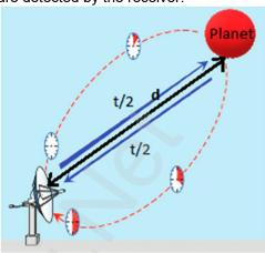
By measuring the time interval between the instants the radio waves are sent and received, the distance of the planet(d) can be determined
