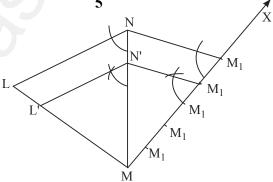
5. Construct a triangle similar to a given triangle ABC with its sides equal to  $\frac{6}{5}$  of the corresponding sides of the triangle ABC (scale factor  $\frac{6}{5} > 1$ ). SEP-20
