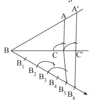
6. Construct a triangle similar to a given triangle PQR with its sides equal to  $\frac{7}{3}$  of the corresponding sides of the triangle PQR (scale factor  $\frac{7}{3} > 1$ ).
