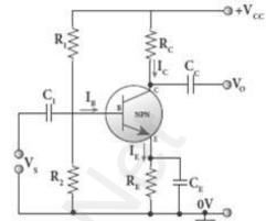
The coupling capacitor CC is used to couple one stage of the amplifier with the next stage while constructing multistage amplifiers.  $V_S$  is the sinusoidal input signal source applied across the base-emitter. The output is taken across the collector-emitter.  $I_c = \beta I_B$
