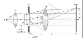
different points on the slit can be treated as parallel lines, making and angle  $\theta$  with the normal 'CO'.
