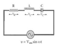
Consider a circuit containing a resistor of resistance 'R', a inductor of inductance 'L' and a capacitor of capacitance 'C' connected across an alternating voltage source.
