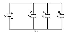
The equivalent capacitance of capacitors connected in parallel is equal to the sum of the individual capacitances.
