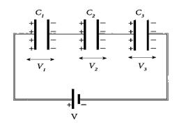
The inverse of the equivalent capacitance  $C_S$  of three capacitors connected in series is equal to the sum of the inverses of each capacitance
