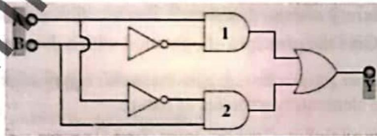
In the combination of the following gates, write the Boolean equation for output Y in terms of inputs A and B.
