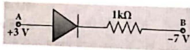
Consider an ideal junction diode. Find the value of current flowing through AB is
