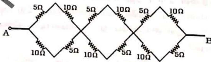
Determine the effective resistance of the given circuit between points A and B.
