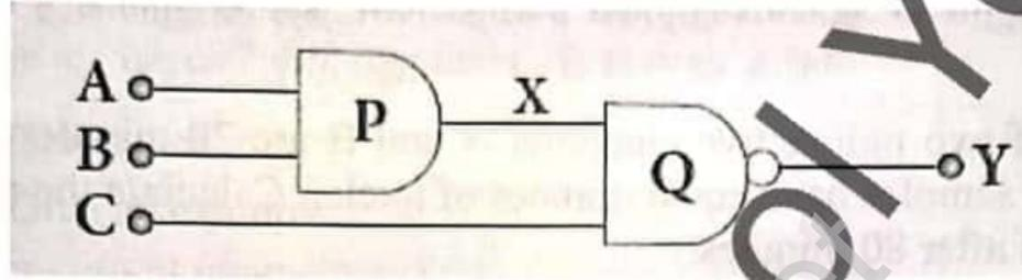
What is the output Y in the above circuit, when all the three inputs A, B, and C are 0 ?
