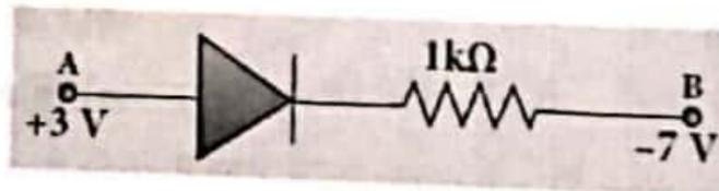
Consider an ideal junction diode. Find the value of current flowing through AB is
