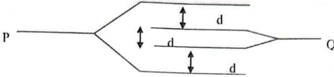
The resultant capacitance of four plates, each is having an area  $A$ , arranged as shown above, will be (plate separation is  $d$ )
