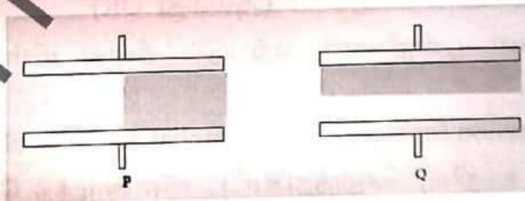
Capacitors P and Q have identical cross sectional areas A and separation d. The space between the capacitors is filled with a dielectric of dielectric constant  $\epsilon_r$  as shown in the figure. Calculate the capacitance of capacitors P and Q.
