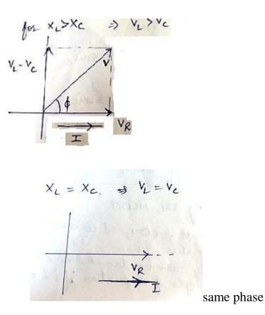
(c) Acceptor circuit: Series LCR circuit
