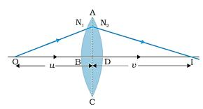
When a ray refracts from a lens (double convex), in above figure, then its image formation can be seen in term of two steps :
