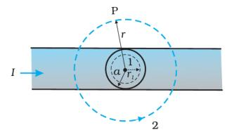
(a) Consider the case r > a. The Amperian loop, labelled 2, is a circle concentric with the cross-section. For this loop,  $L = 2 \pi r$
