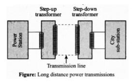
The large-scale transmission and distribution of electrical energy over long distances is done with the use of transformers. The voltage output of the generator is stepped-up. It is then transmitted over long distances to an area sub-station near the consumers. There the voltage is stepped down. It is further stepped down at distributing sub-stations and utility poles before a power supply of 240 V reaches our homes.
