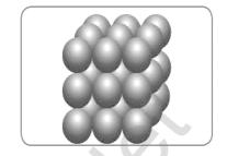
above and one below and hence the coordination number of the sphere in simple cubic arrangement is 6.
