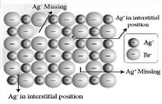
Small Ag<sup>+</sup> ion leaves its normal site and occupies an interstitial position.
