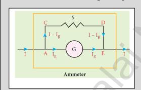
In order to increase the range of an ammeter n times, the value of shunt resistance to be connected in parallel is
