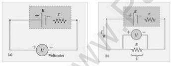
• When the electric circuit is open, the reading in voltmeter(v), is equal to the electro motive force ( $\varepsilon$ )
