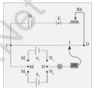
• Balancing length  $l_1$  is determined when key  $K_2$  is open. According to principle of potentiometer.
