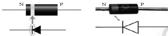
Figure (a) PN junction diode and its symbol (Silver ring denotes the negative terminal of the diode)
