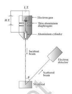
are then accelerated due to the potential difference between the filament and the anode aluminium cylinder by a high tension (H.T.) battery.
