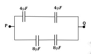
$4\mu F$  and  $4\mu F$  capacitors are in series, their effective capacitance is
