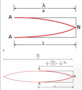
let L be the length of the tube and the wavelength of the wave produced. For the fundamental mode of vibration, we have
