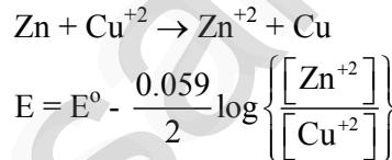
Lesser the value of  $\frac{[\text{Zn}^{+2}]}{[\text{Cu}^{+2}]}$  greater will be the  $E_{\text{cell}}$
