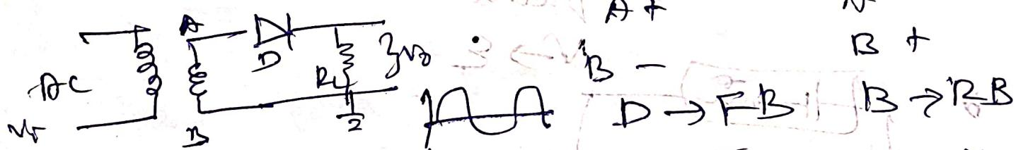
$$\text{Efficiency } \eta = \frac{\text{O/P DC power}}{\text{I_P AC power}} \approx 40.6\%$$
