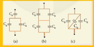
4. For the given capacitor configuration (a) Find the charges on each capacitor (b) potential difference across them (c) energy stored in each capacitor
