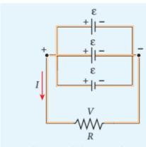
Cells in parallel (circuit diagram)
