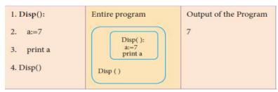
• On execution of the above code the variable a displays the value 7, because it is defined and available in the local scope.
