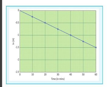
Decomposition of hydrogen peroxide catalysed by I<sup>-</sup>
