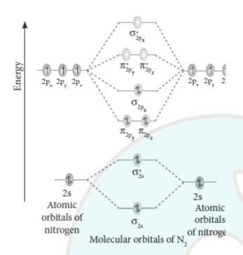
Molecular orbital diagram of nitrogen molecule (N<sub>2</sub>)
