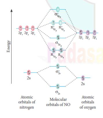
Molecular orbital diagram of Nitric oxide molecule (NO)
