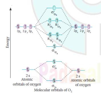
Molecular orbital diagram of oxygen molecule (O<sub>2</sub>)
