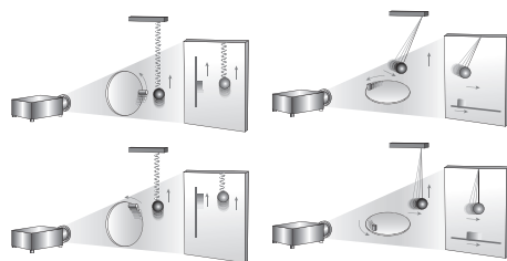
Motion of spring mass (or simple pendulum) related to uniform circular motion
