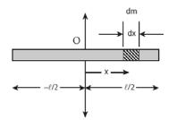
3) We take an infinitesimally small mass (dm) at a distance (x) from the origin. The moment of inertia (dl) of this mass (dm) about the axis is,
