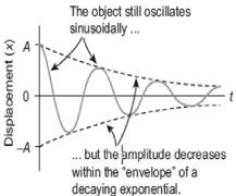
4) The motion of the oscillator is said to be damped and in this case, the resistive force (or damping force) is proportional to the velocity of the oscillator.
