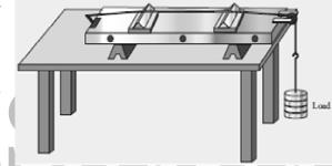
5) Two adjustable wooden knives are put over the board, and their positions are adjusted to change the vibrating length of the stretched wire.
