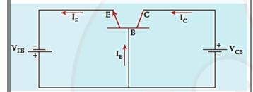
54. Draw the schematic circiut diagram of CE configuration.
